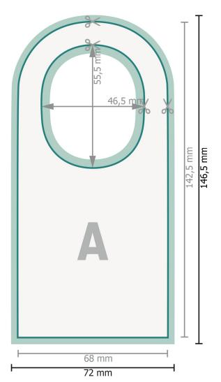
Please remove the die line fom the download template before generating your printfiles. Please provide a second file (view file) to specify the position of the die line. Dataformat (incl. 2 mm bleed): 7,2 x 14,65 cm
